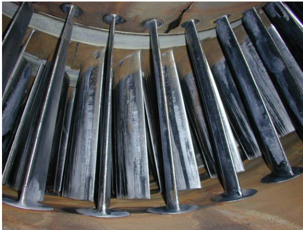
Fouled GT engine compressor
